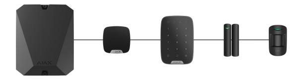
For the **Beam (Radial)** topology, be sure to install a 120 Ohm terminating resistor at the end of the line (included in the hub complete set). The terminating resistor is connected to the signal terminals of the last device in the line.
